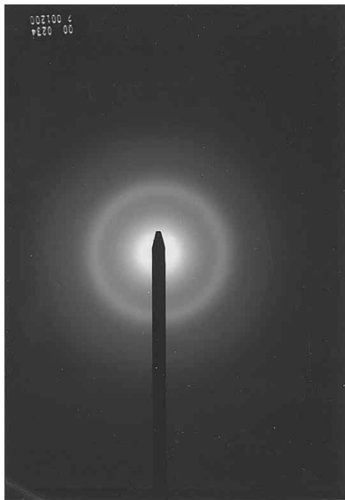
Fig. 3. An Electron Diffraction Pattern of a Mineral Deposit Demonstrating the Characteristic Crystalline Structure of Hydroxyapatite
